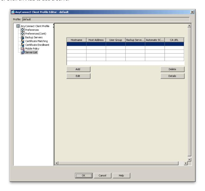
9. Enter the FQDN of your Cisco ASA VPN exposed end-point in the **Hostname** and a hostname or IP Address in the **Host Address**
