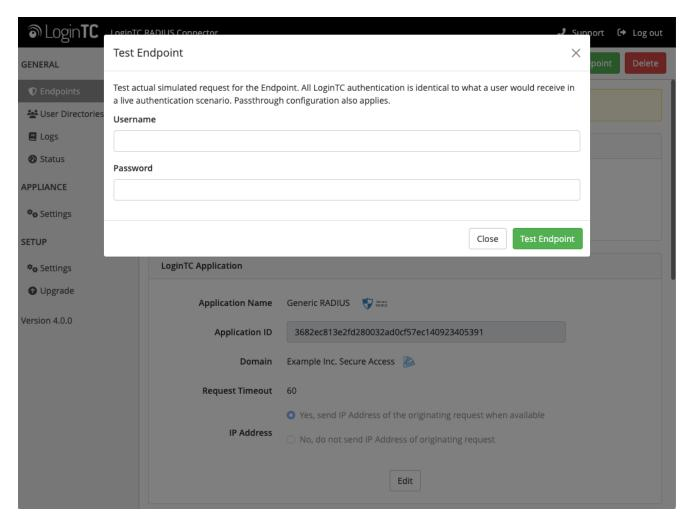
Enter a valid username and password; if there is no password leave it blank. A simulated authentication request will be sent to the mobile or desktop device with the user token loaded. Approve the request to continue:
